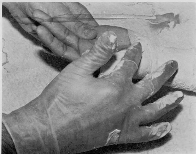
Photo 7. RTV-11 compound is smoothed evenly over the gauze.
