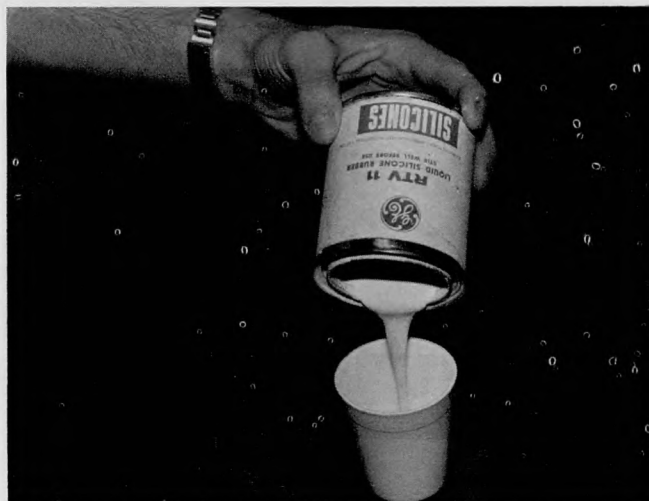
Photo 5. RTV-11 compound is poured into cup and curing agent added.
